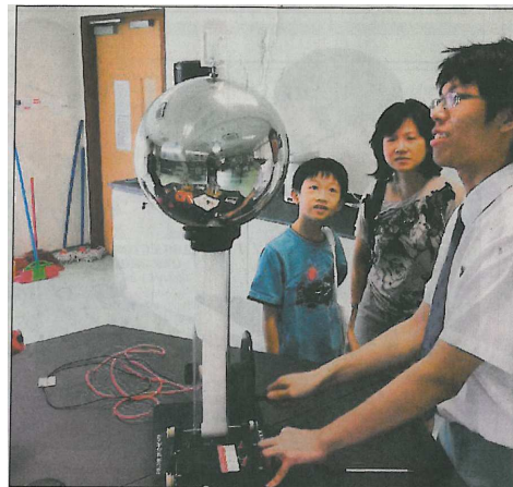
An NUS High student demonstrating a Van de Graff generator - which generates high voltage within its metal sphere - at an open house last month. PHOTO: NUS HIGH
